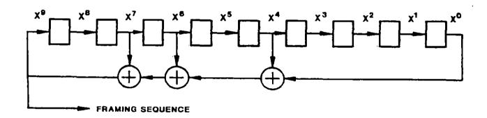
FIGURE B-5. Framing sequence feedback shift register generator.
