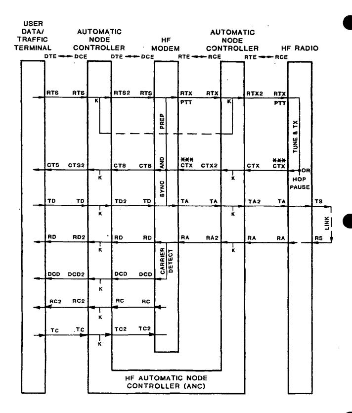
FIGURE 3. An example of equipment interface block diagram.
