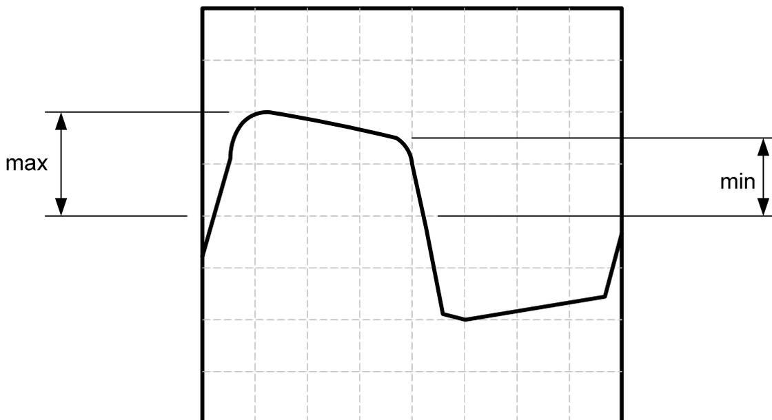
**Figure 4: DCS waveform showing distortion measurement**
