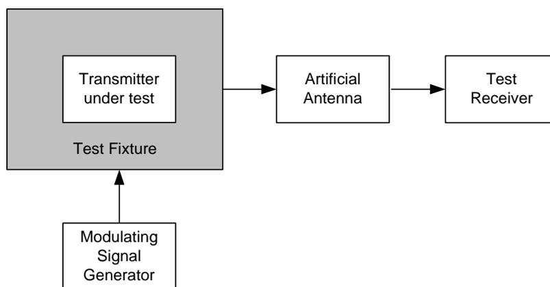
**Figure 3: Measurement arrangement**
