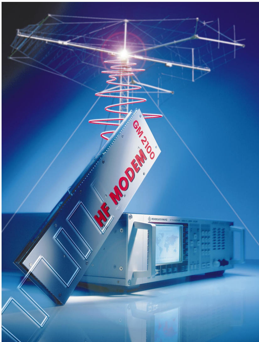
FIG 1 HF Modem GM2100 for shortwave data transmission at up to 5400 bit/s
